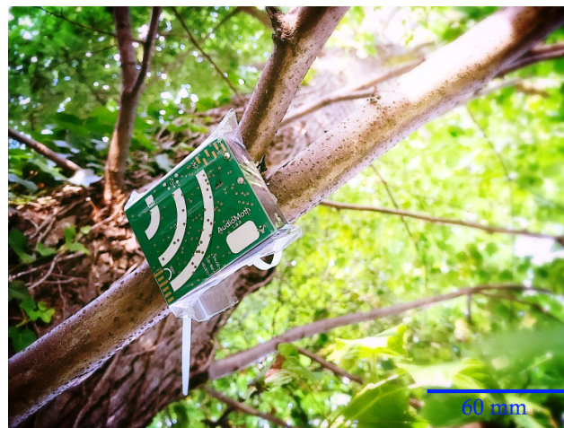
Figure 1. AudioMoth: a low-cost, low-power acoustic monitoring device developed for a wide variety of conservation projects, deployed on a tree in a grip-sealed bag using a cable tie.
