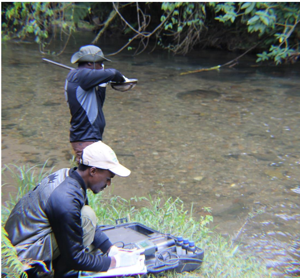
Figure 6. Collecting in situ physicochemical parameters using a HANNA multiparameter probe meter. Photo by J. Ndimulodi.
