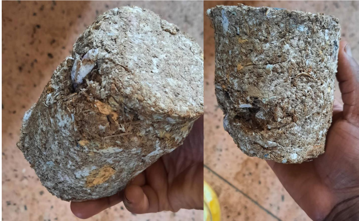
Figure 16: A sample of a paper log briquette produced by the local community members for fuel use
