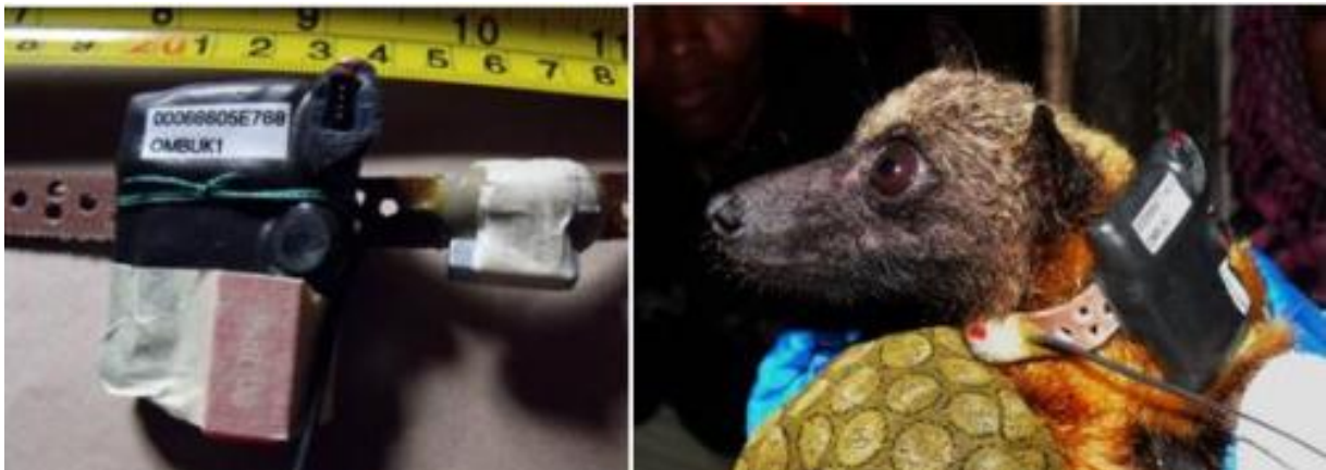
Fig.5. Left: GPS and RF tag on a collar. Right: collar attached to P. rufus .
