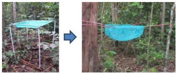
Figure 2. Modification of seed trap design
