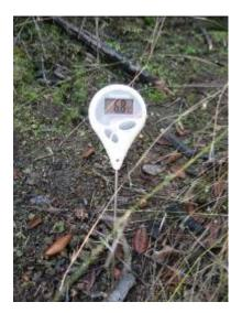
As it was stated on the basic Final Report, only the ground temperature was measured. The field protocol consisted in the temperature measurement of the substratum shade using a ground thermometer (measurement range: -10 to 200°C) in 50 points of each matrix table box. The data for each box were averaged out.
