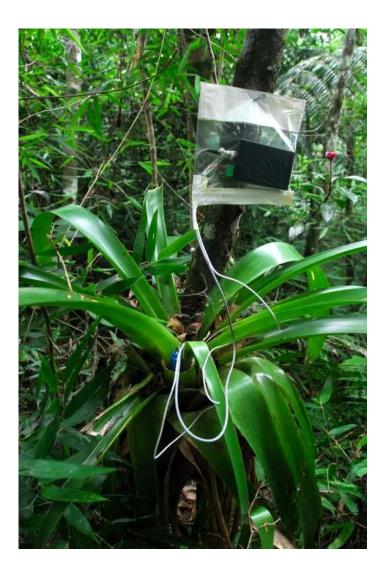
Figure 6. PHTEMP101 Data Logger *in situ* with pH and temperature probes extending into bromeliad tank (*Tillandsia guatemalensis*). The unit is sealed within a plastic bag to protect the electrical components from precipitation and humidity.
