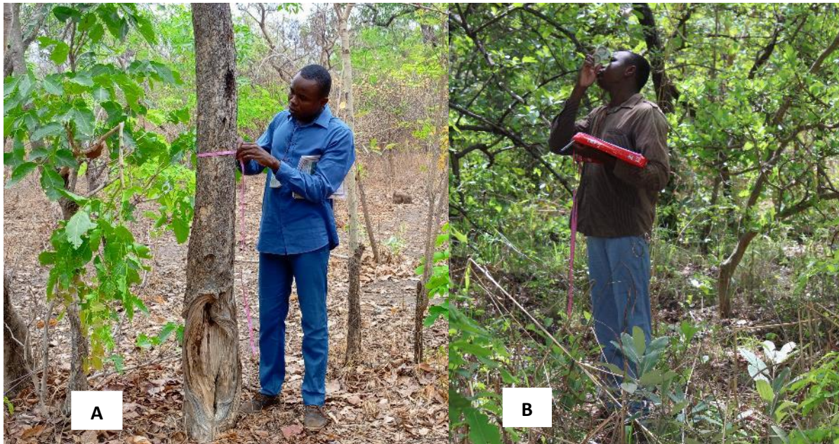
Photo 1. (A) Measuring dbh 1.3m using a Ruban pi, (B) Measuring sight angles using a Clinomètre for height estimation.
