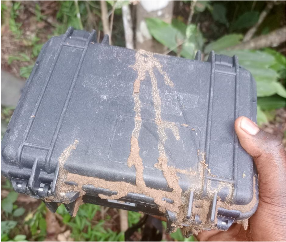
Termite infested device cleaned during monitoring.
