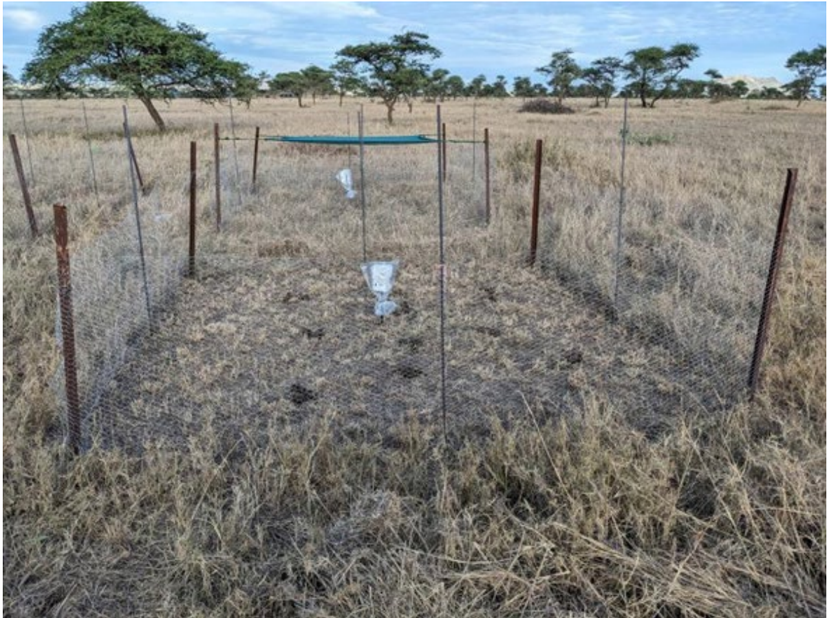
Figure 3: Established cages with introduced dung piles and temperature and humidity sensors (covered in white containers and plastic bags).
