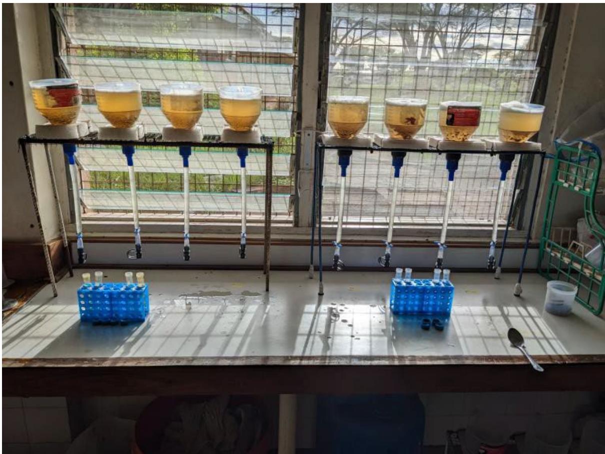
Figure 6: Filtration of gastrointestinal larvae through funnel filters into test tube for further processing prior to counting of larvae.
