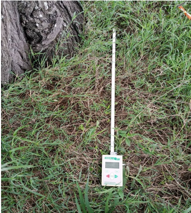
Figure 3; Light meter for assess variation of sunlight (effect of tree shade) between outside tree canopy and under tree canopy.
