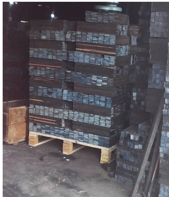
Figure 6 : This picture shows Diospyros crassiflora bundles of timber already sawn inside a house converted into a sawmill. In this house, only ebony wood is transformed. Taking pictures is strictly prohibited.
