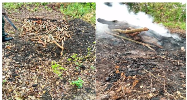
Figure 9. Charcoal kiln construction. Figure 10. A fresh charcoal kiln.
