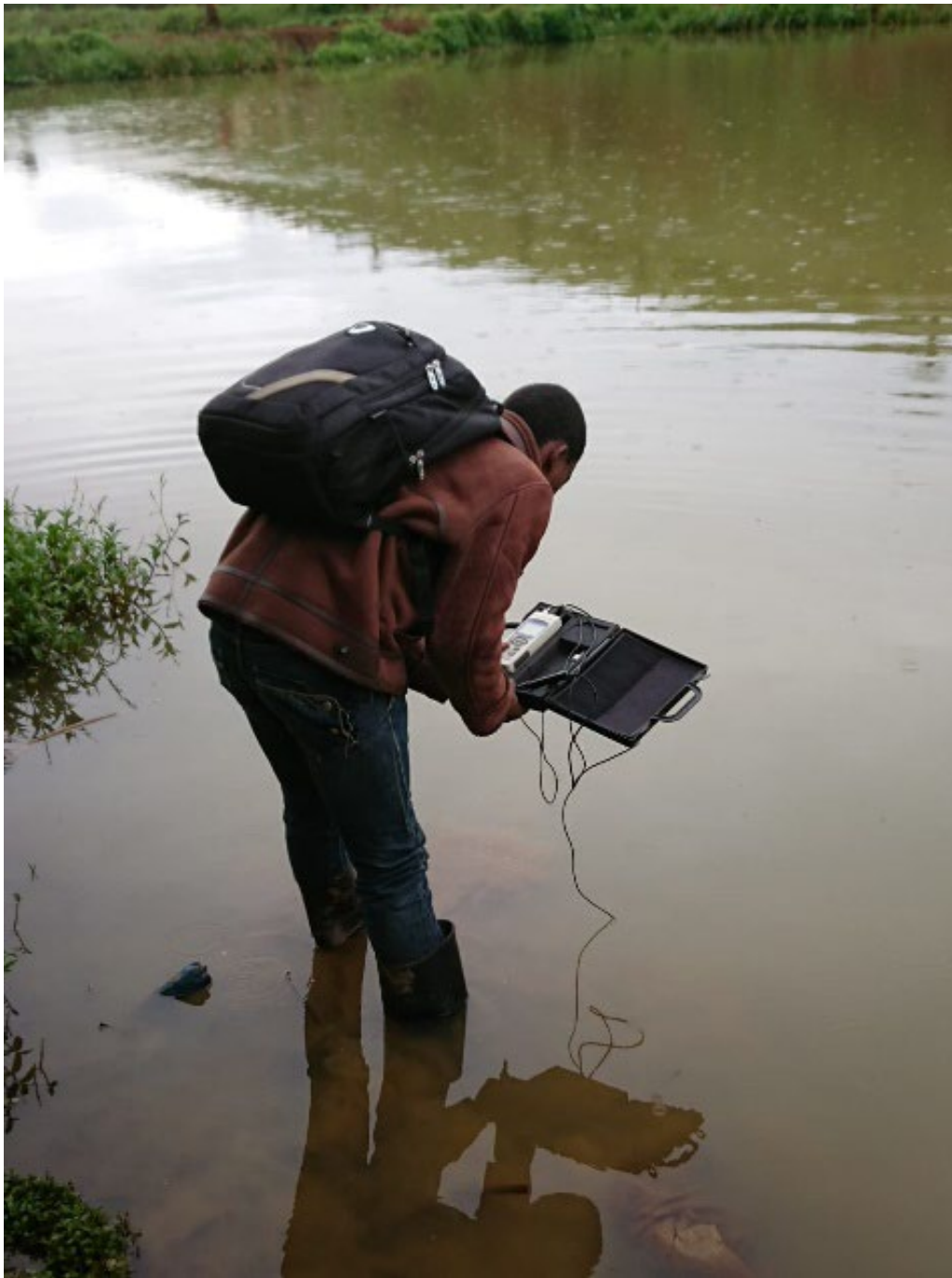
Figure 5: Water parameter collection using a multiparametric probe.
