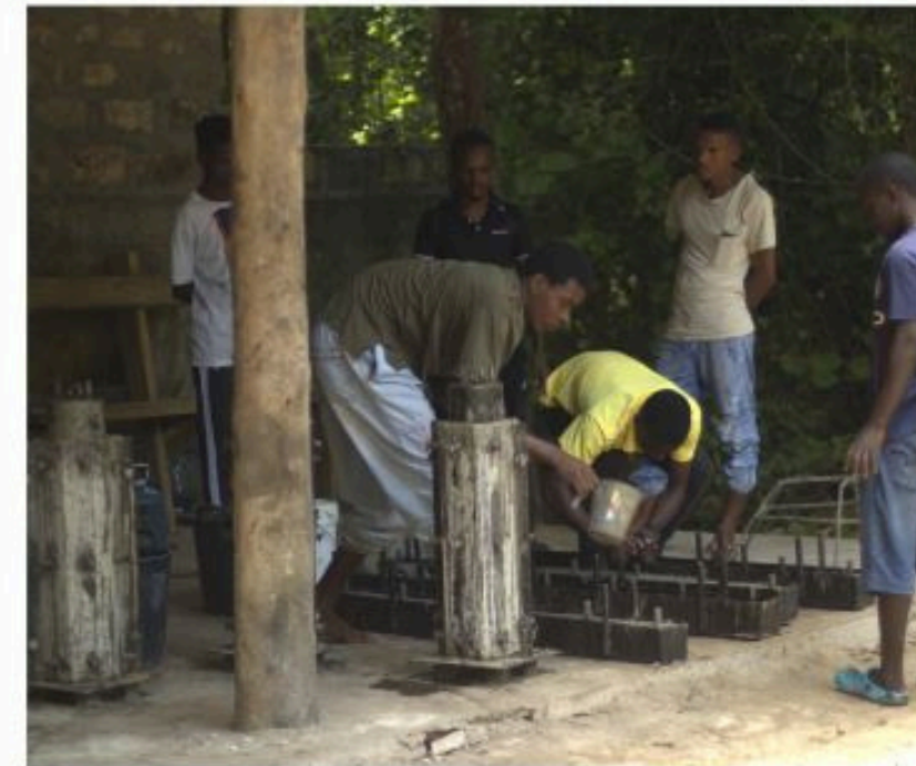
Members of a Beach Management Unit (BMU) make artificial reefs at the training workshop in Kwale County, Kenya's coast.
