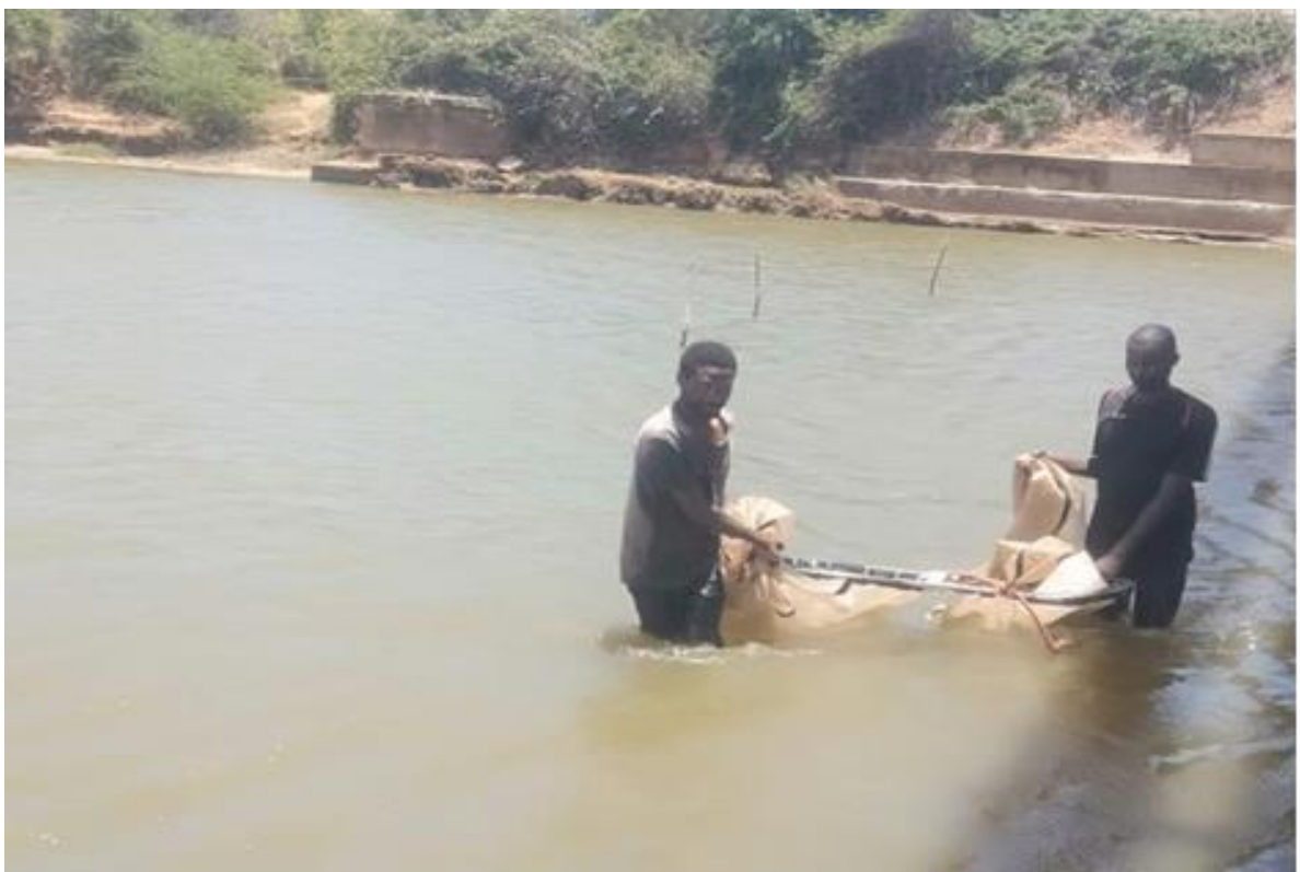
Figure 3: Bongo net deployment in River Sabaki water column for plastic litter monitoring.
