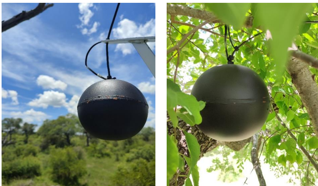
Figure 3. Black bulbs installed in different microsites to measure operative temperatures, used to describe environmental temperatures experience by ground-hornbills in different microsites. Left: in a tree exposed to full sun. Right: in a tree with shade.
