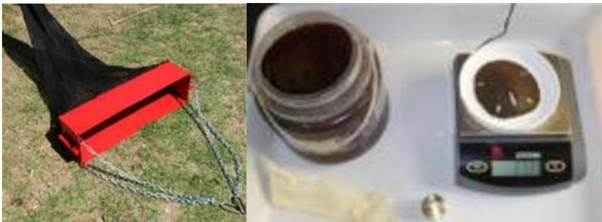
Left: Dredge to take samples from macrobenthos. Right: Scales bought to register the invertebrates' weight.
