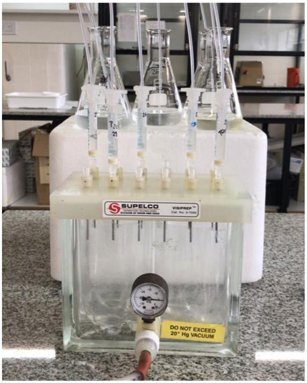
Extracting water samples by SPE in the laboratory.
