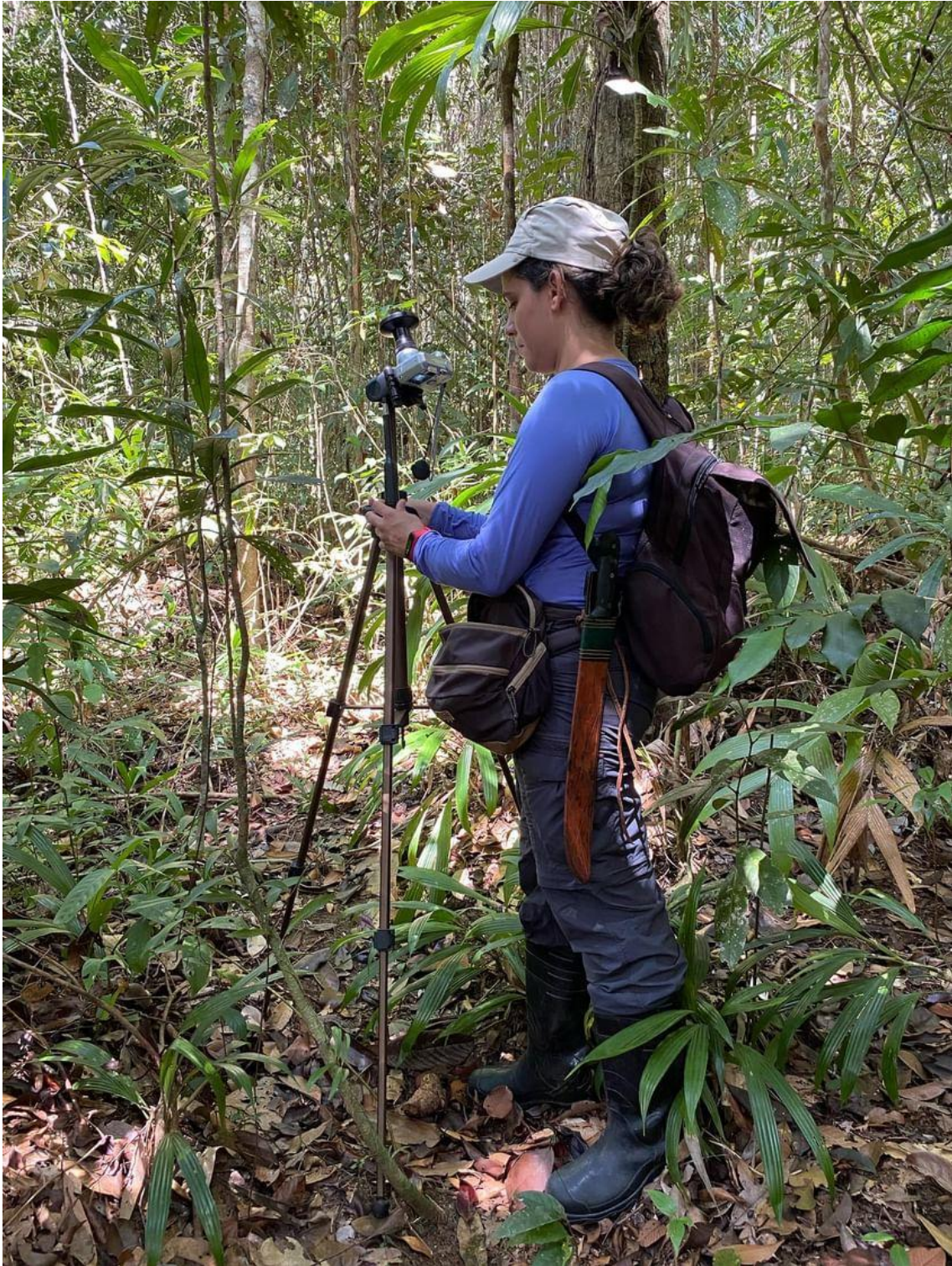
Figure 7: Taking canopy hemispherical photos using a fisheye lens © Ana Flávia do Nascimento.
