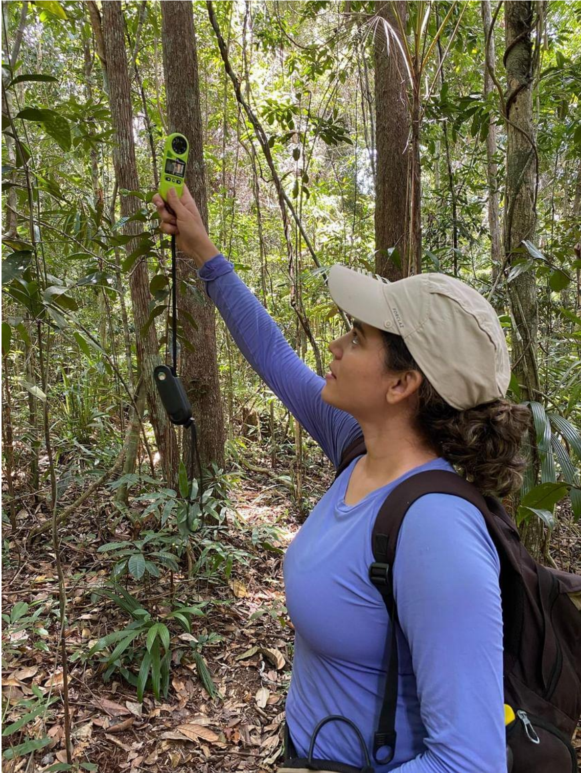
Figure 6: Collecting temperature and humidity with a portable weather station © Ana Flávia do Nascimento.
