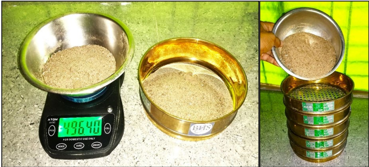
Weighing of dried sand sample (left) and pouring of sand sample to test sieves. © Pawan Pareek.
