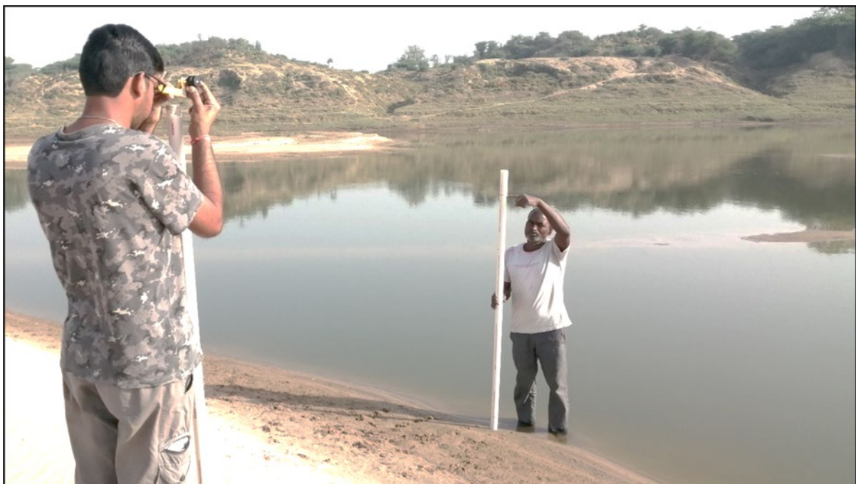
Measuring the slope of nesting sand banks using Abney level. © Shishubhan Singh.
