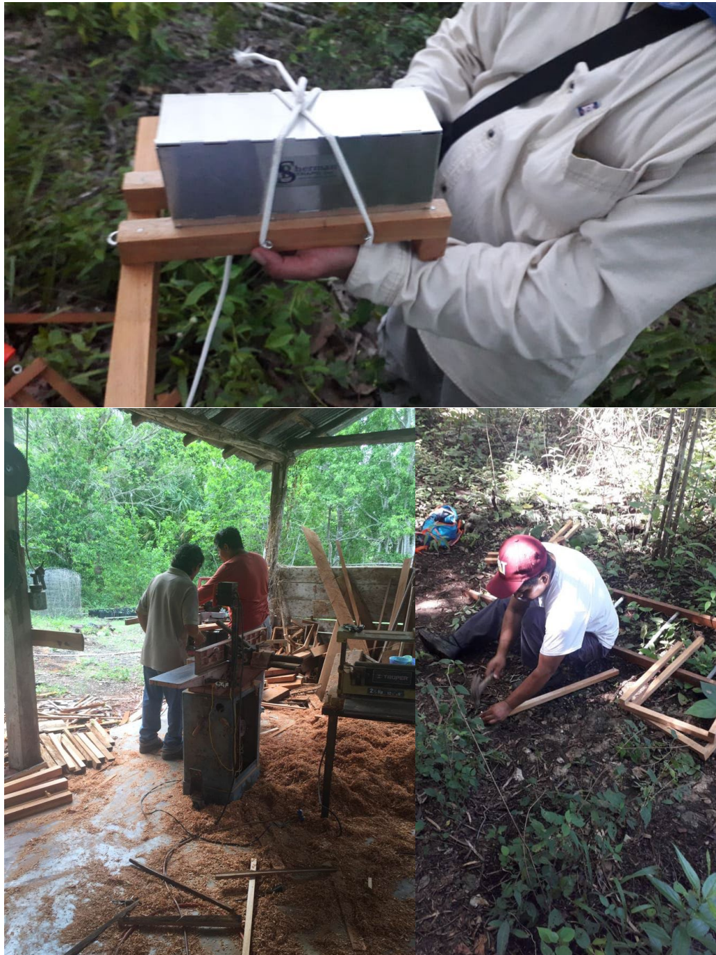
Figure 1: Elaboration of the structures to install Sherman traps in the canopy
