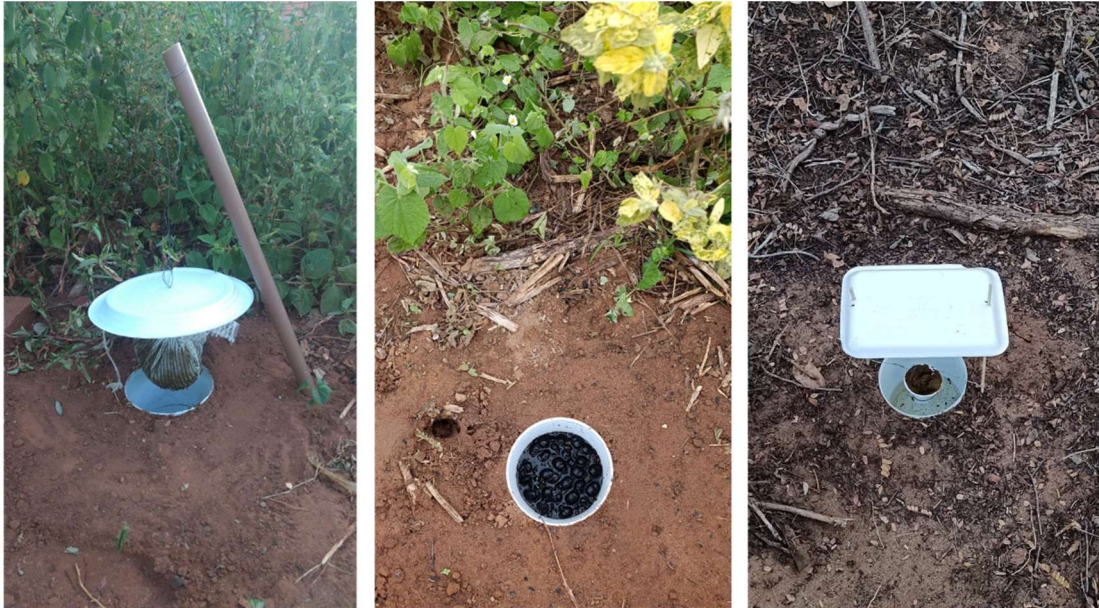
Figure 2 a, b, and c - Pitfall traps baited installed for dung beetle sampling. Figure 2b pitfall traps after 24 hours.
