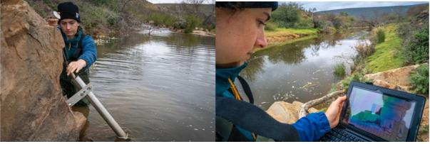
Left: Retrieving the level logger from the Biedouw River prior to downloading the data. Right: Visualising the data from the level logger installed in the Biedouw River. The red curve shows temperature. The blue curve shows pressure (which can be converted into flow). © Dr Jeremy Shelton.
