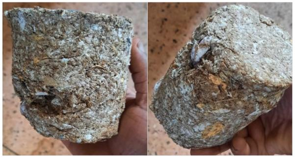
Figure 2: A sample of paper log briquettes, a cost-effective, eco-friendly alternative fuel source.
