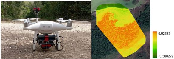
Figure 4. The multispectral camera mounted to a Phantom drone (on the left) can be used to create orthomosaic imagery of the Bacalar forest, e.g., showing NDVI values of present vegetation. Such information might be useful to infer water stress of trees and relate it to the presence of superficial and subterranean water sources.
