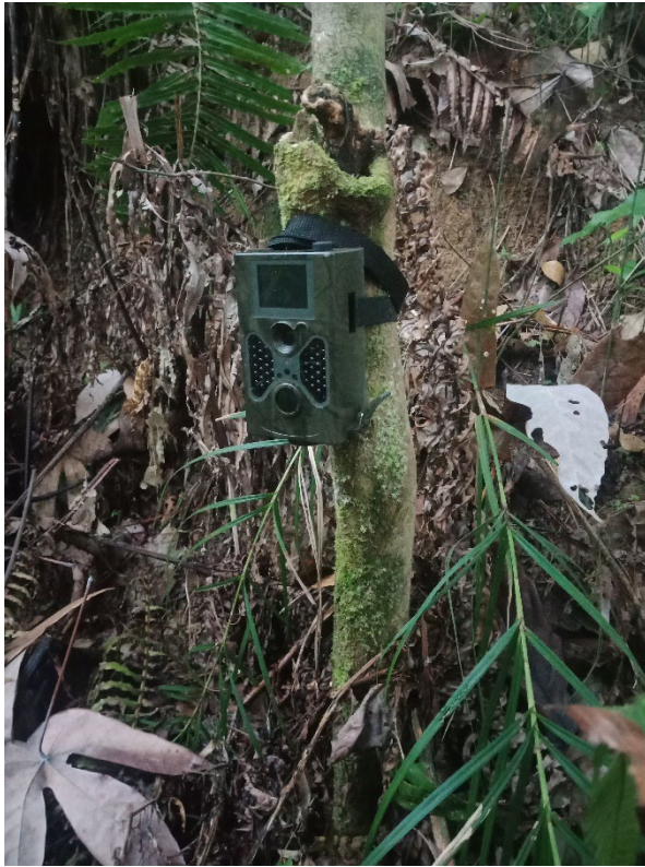
Picture 3 & Picture 4. These pictures show the design used in positioning the camera traps onto the tree stands, which are located around 2.0 to 3.0 m away from the areas-in-interest. The height from ground and distance from the area-in-interest respectively are varied between each sampling points, mainly to make sure that all the deployed camera traps are able to capture clear footage of terrestrial mammals with different sizes. Any obstacles that are potentially blocking the field of vision of the camera trap are removed. These pictures are taken using my own phone on 29 th September 2022.
