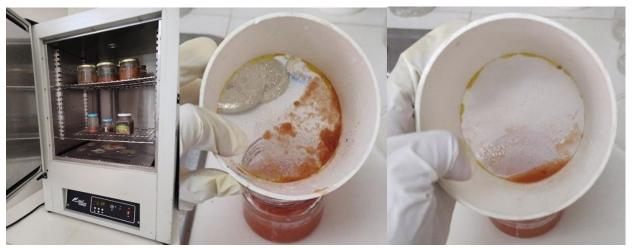
Figure 1: Samples in the organic matter digestion process. Figure 2. Sample filtering through two different meses.
