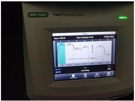
Thermocycler setting during Polymerase chain reaction (PCR) of my samples in laboratory of NTNC, Chitwan.
