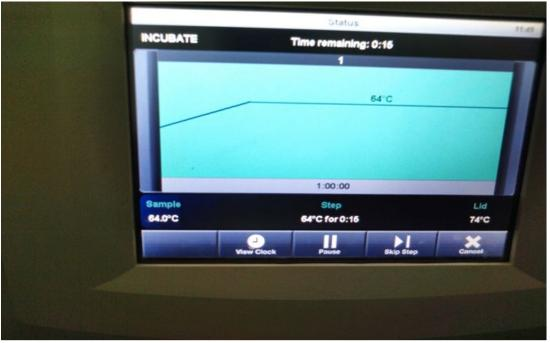
Setting of Incubator for LAMP test of my samples.
