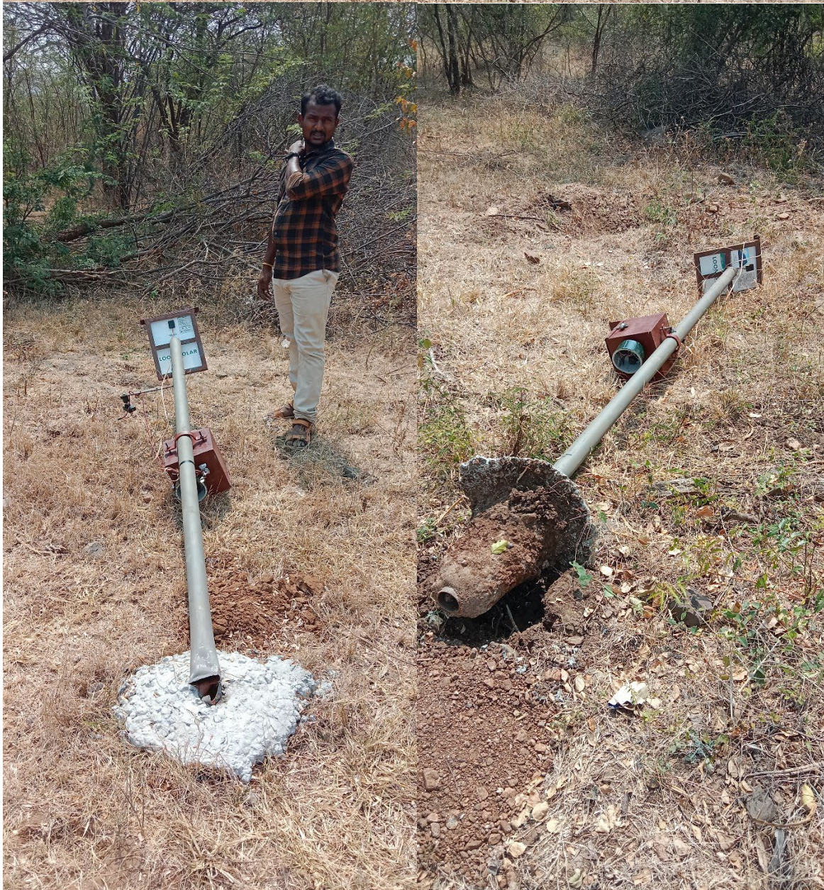
A receiver unit knocked down by elephant (top & bottom left) and a transmitter pole knocked down by bison (bottom right).
