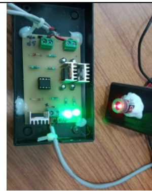
Testing of transmitter PCB functionality
