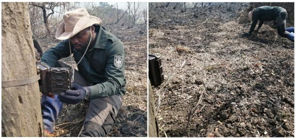
Figure 3: (a) installation of a camera trap on a tree to monitor a potential giant pangolin / aardvark location (b) crawling test to check correct functioning and correct angling of camera traps.
