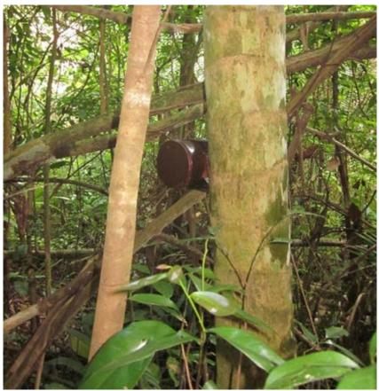
Figure 1. AudioMoth acoustic sensor inside its protective case deployed in Tapir Mountain Nature Reserve.
