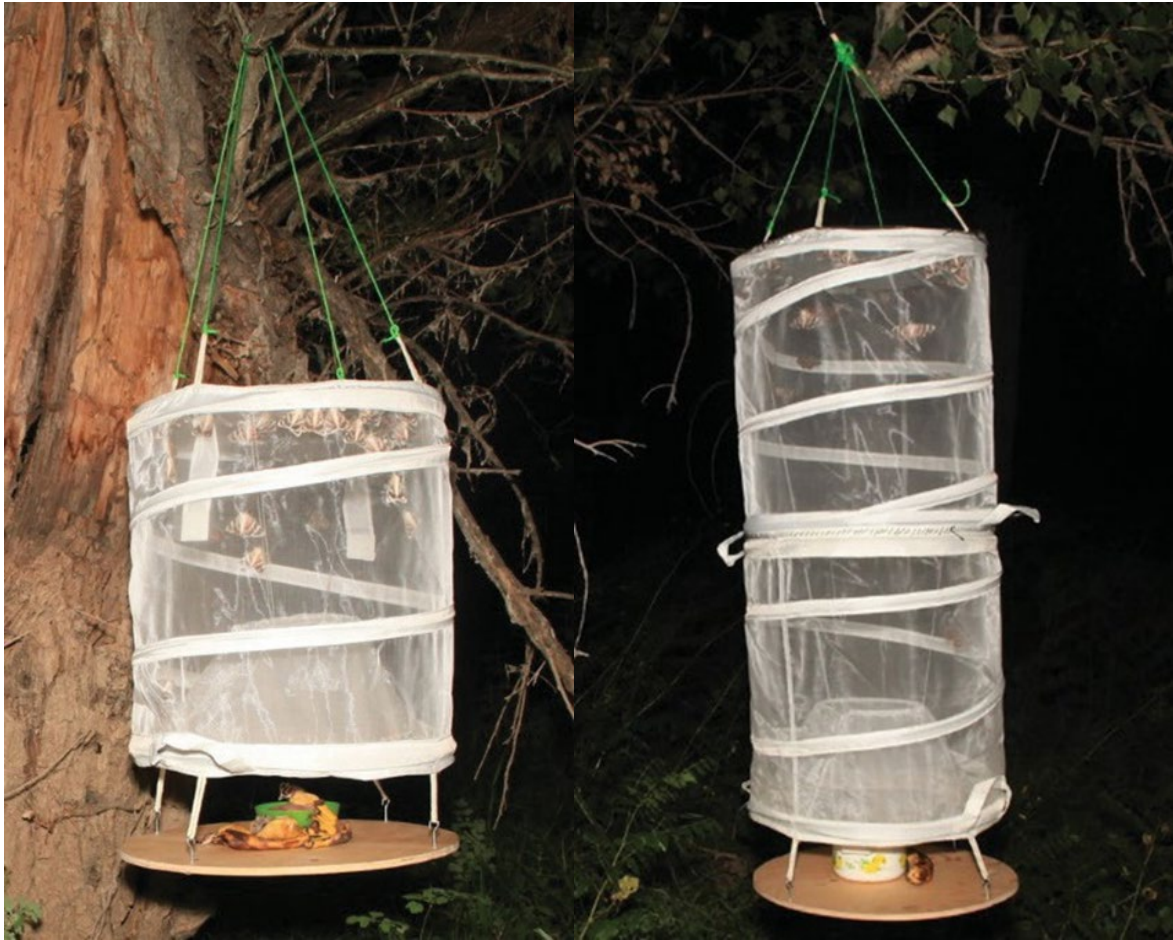
Cage traps with aromatic bait made from wine, sugar and overripe bananas.
