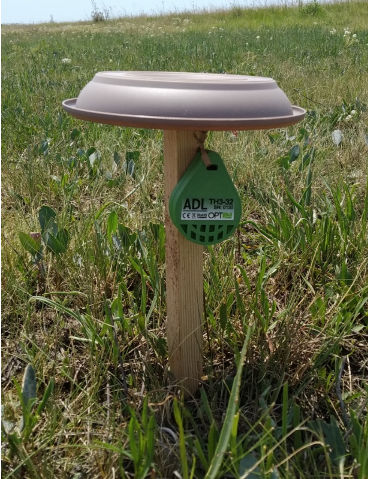
Ambient data logger installed in the field.
