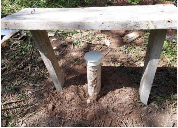
Photo 2. A freatimeter installed inside the forest.
