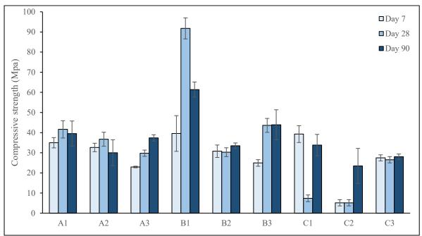
Fig. 3. Compressive strengths of different mix designations on day 7, 28 and 90 (%).
