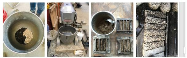
Fig. 1. Eco-concrete produced with quarry dust and crushed shells as coarse aggregate.
