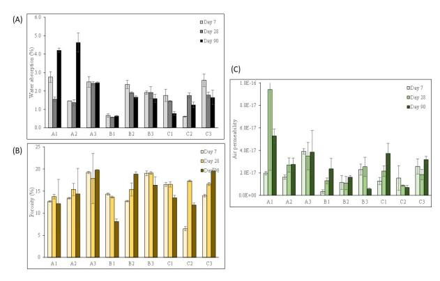
Fig. 5. Tests conducted in 7 days, 28 days and 90 days on the different mix designations (%): (A) Water permeability, (B) Porosity, and (C) Air permeability.
