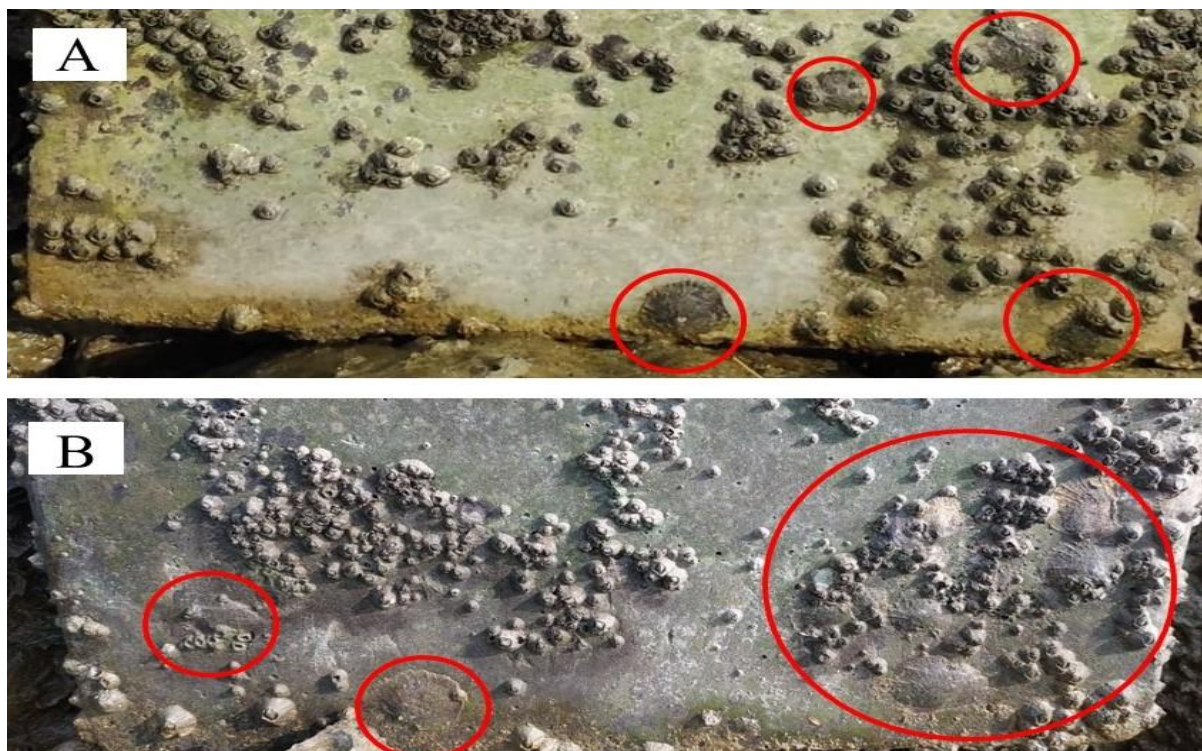
Figure 11. (A) Saccostrea cucullata on the blank Portland cement panels (BC) and (B) on the blank eco-concrete panels (BE).
