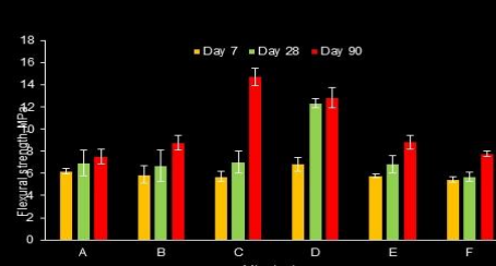
Figure 3. Tensile strength performance of each concrete mix design. Noted that "A" is referred as conventional Portland concrete.
