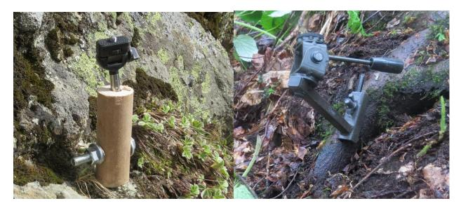
Photo 14; 15: Self-made camera trap mount (left) and HME Camera trap mount (right)
