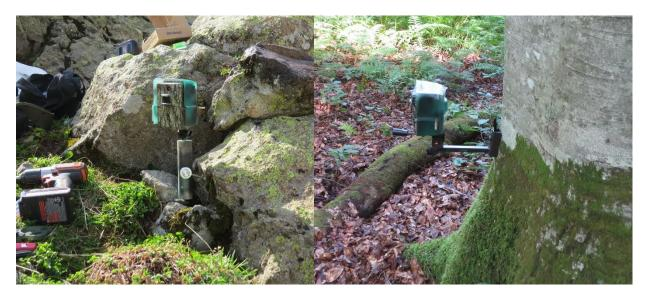
PHOTO 16; 7: CAMERA TRAPS IN WORKING CONDITIONS, ON HAND-MADE (LEFT) AND HME (RIGHT) MOUNTS.
