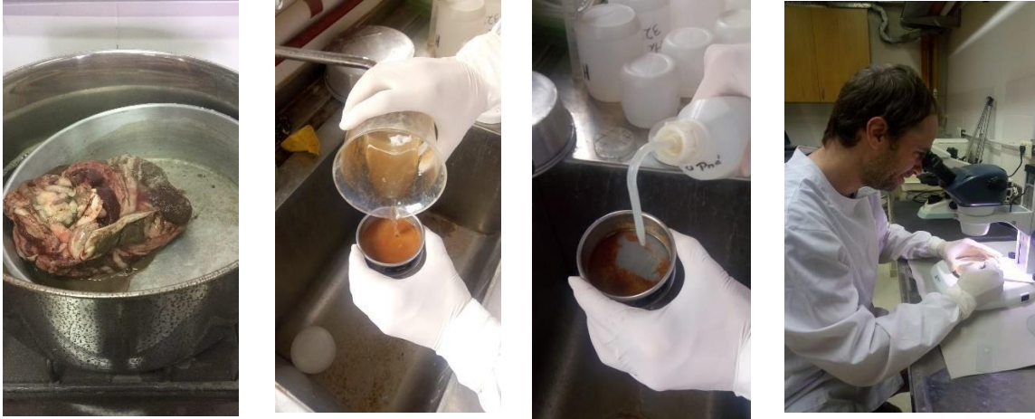
Figure 2. Samples (fish digestive tract) processing. From the left to the right: removal digestive tract, stomach content after 30% hydrogen peroxide digestion, sieving through a stainless steel (350 \mu\text{m} mesh size), microscope examination.
