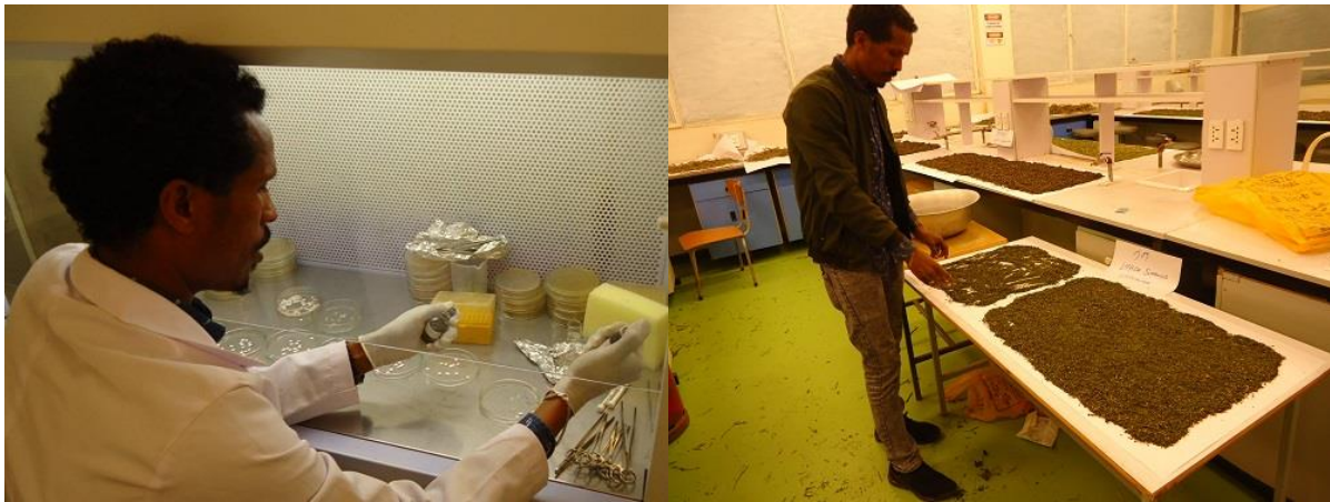
Left: Plant specimen extract application against pathogens at Laminar hood. Right: Drying specimen for extraction at room temperature.
