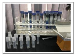
Figure 1. Sampling kits consisting of cryovials (2ml) and falcon tubes (15ml)
