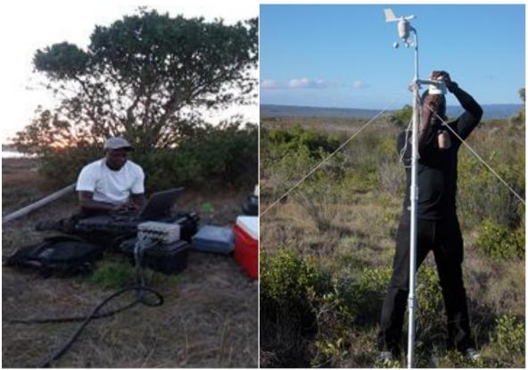
Left: Set up of multiple microphone arrays to record echolocation calls of free flying bats in a foraging site in Fynbos biome at Dehoop Nature Reserve. Right: A portable weather station to record weather parameters (temperature, relative humidity, atmospheric pressure and wind speed) at the same while recording echolocation calls.
