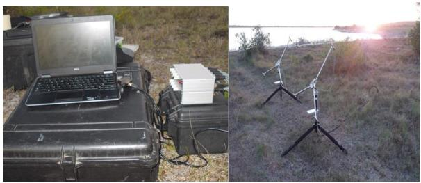
Left: Ultrasound gate receiver connected to laptop. Right: Set up of multiple microphone arrays to record echolocation calls of free flying bats in a foraging site in Fynbos biome at Dehoop Nature Reserve.
