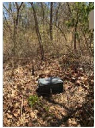
Figure 1. Manual chambers used in the grassland (left) and the forest (right) to measure Greenhouse Gas Emissions in the soil.
