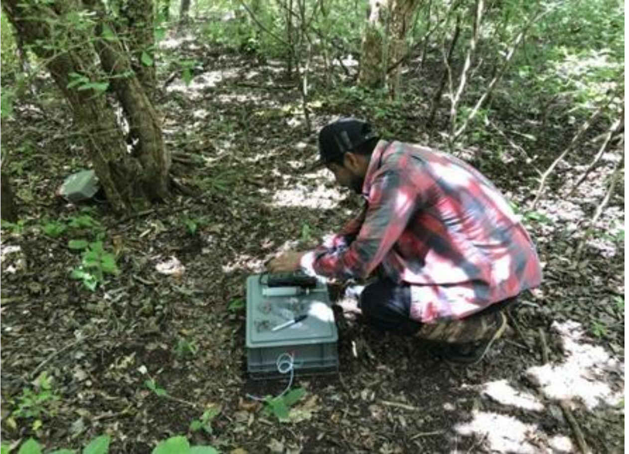
Figure 3. Assistants of the project collecting gas samples and data from soil sensors.
