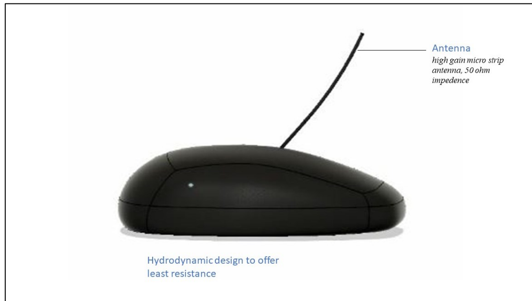
Fig 6: CAD design of the tag housing with the antenna
