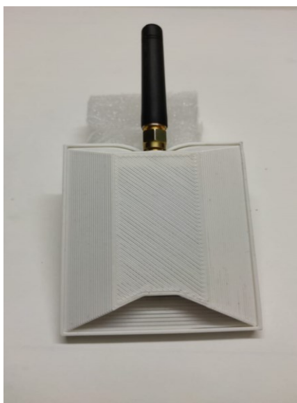
Fig 8: Hand-held receiver to actively look for signals from tag units. The receiver can be coupled to a smartphone through Bluetooth and the data can be downloaded using a dedicated app
