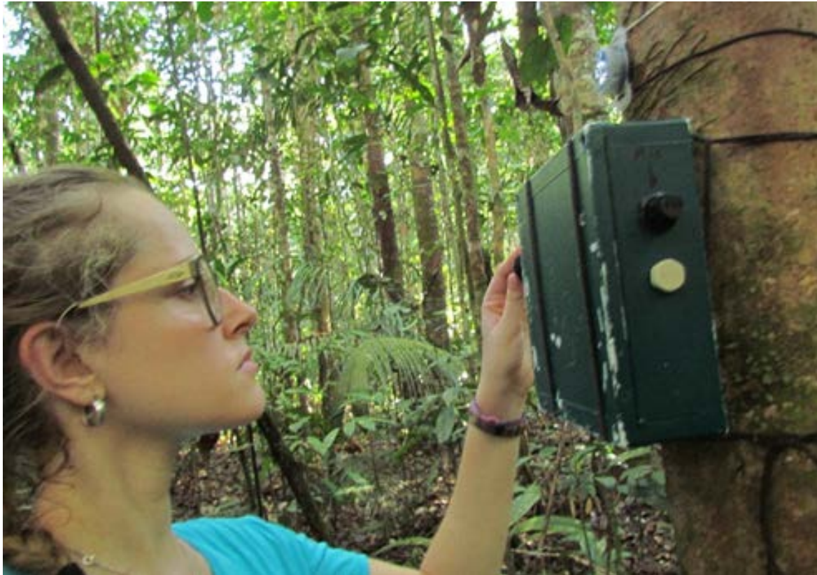
Fig 3. The installation of ultrasound recorder with data loggers that measure air temperature (up) in a continuous forest of Cabo Frio camp in BDFFP areas (Presidente Figueiredo – AM – Brazil). Giulliana Appel
