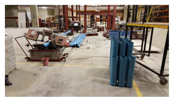
The materials needed for the water purification system are PVC pipes 110 mm and 160 mm diameter. The lengths needed were 60 m and 20 m for the 110 mm and 160 mm diameter pipes respectively. Using a table bandsaw the PVC pipes were cut into the correct lengths. It was established that the optimal depth of each silo is 500 mm, to allow for plant growth, water permeability and a gravel and sand filter with the chamber, above the drainage pipe.
