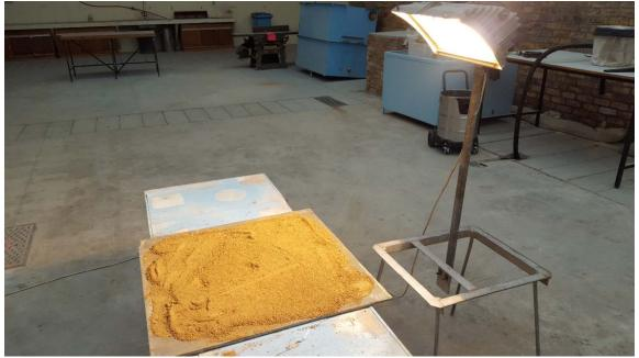
The soil is currently undergoing a soil classification test to establish the content clay, silt and sand. In the above image the soil is dried, which is important when measuring the soil's exact mass. The soil is then ready for a sieve analysis.
