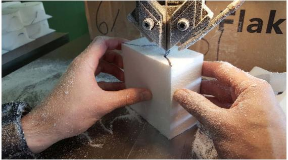
Creating an Iso-Board drainage holster for every silo, using a band saw and carefully marked measurements.
