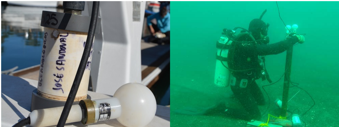
Left: Light sensor installed at site prior to deploying the artificial reefs. Right: We installed some measuring equipment nearby our kelp patches.
