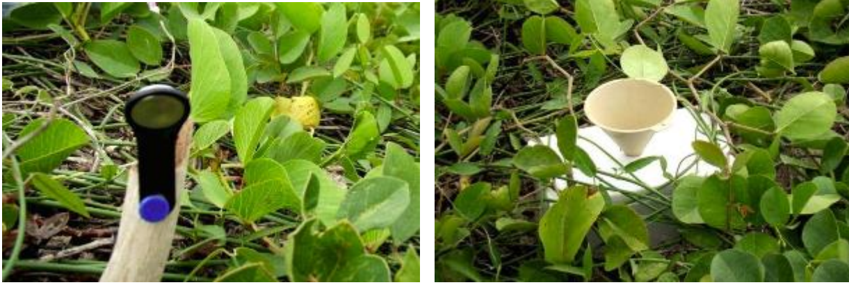
Figure 6. a. Datalogger used to measure temperature and humidity in the environmental stations. b. Set up used to measure rainfall.
